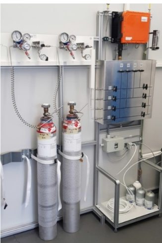
Micro GC system developed for H 2 . Source: meterQ
