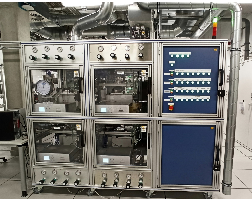
Figure 1: Catalyst test rig at the Max Planck Institute for Chemical Energy Conversion (MPI CEC). Source: Simon Ristig, MPI CEC
